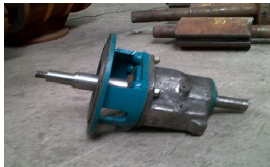
Step 7 –Assembly of Lantern Bracket (Bearing Housing is fitted in Lantern Bracket)
