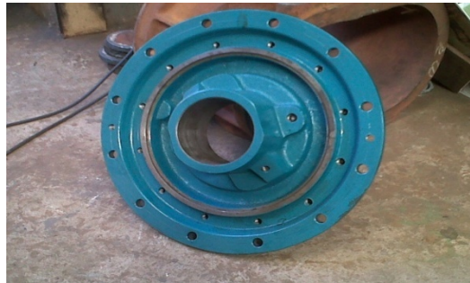
Step 8 – Casing cover (Assembly of Bearing Housing &Lantern bracket is fitted in Casing cover)
