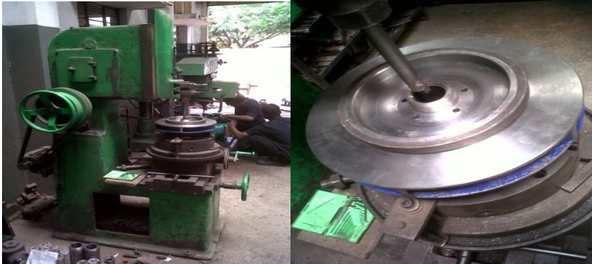
Step 4 – Keyway of required dimension is manufactured on Impeller by slotting machine.
