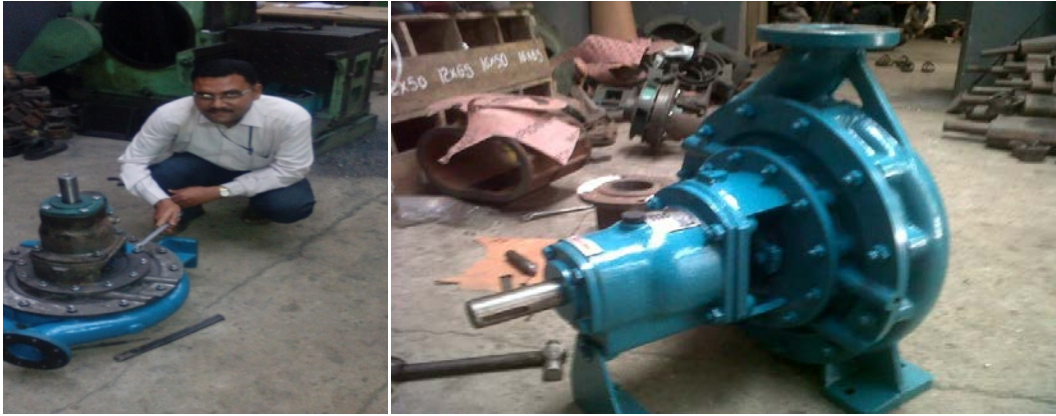
Step 10 - Assembly of Bearing Housing, Lantern Bracket and Casing cover is fitted in Casing Of centrifugal pumps
