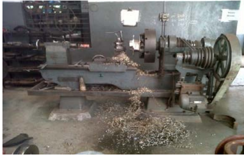
Step 3 – Enclosed Impeller is machined on lathe machine
