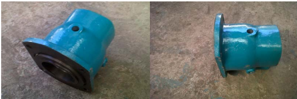
Step 6 – Bearing housing (Shaft & Bearing is fitted in Bearing Housing.)
