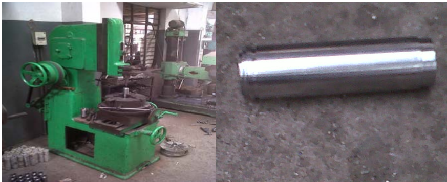
Step 5 – Keyway of required dimension is manufactured on Sleeve by Slotting machine
