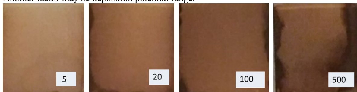
Figure.2 Photographs of coatings fabricated with different scanning speeds.
